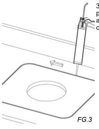
3. Apply a bead of silicone to the perimeter of the hole at the point at which the sink sits on the counter. *FG.3*
